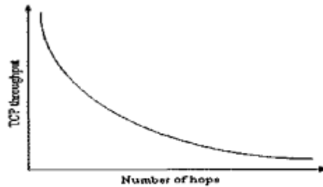
Figure 7.8 – TCP throughput is inversely proportional to the number of hops
